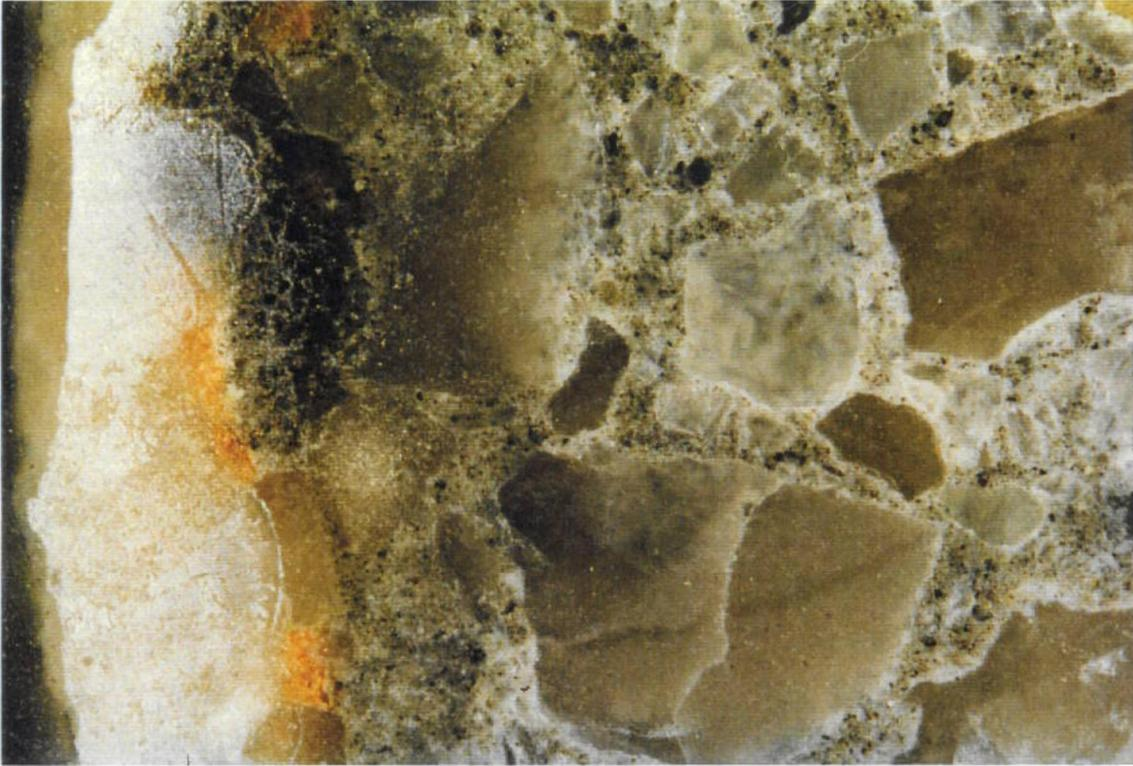
**Image 14:** Corrosion border zone of mortar **K HS 0** with limestone and CEM I 42.5 R HS NA (**unmodified**) after 70 days of storage in pH 1 sulphuric acid, ground, under the microscope. The image width is 2.7 mm (55x magnification).
