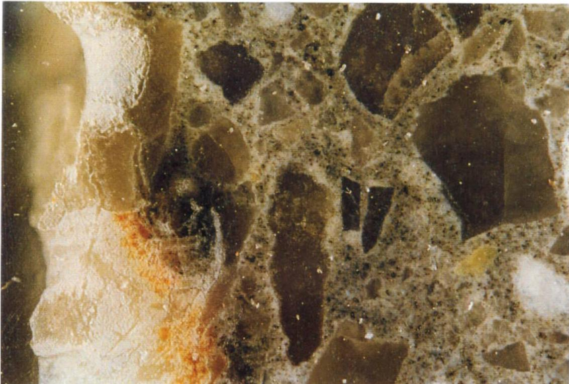
**Image 15:** Corrosion border zone of mortar **K HS 1** with limestone and CEM I 42.5 R HS NA **MOWILITH-modified** after 70 days of storage in pH 1 sulphuric acid, ground, under the microscope. The image width is 2.7 mm (55x magnification).
