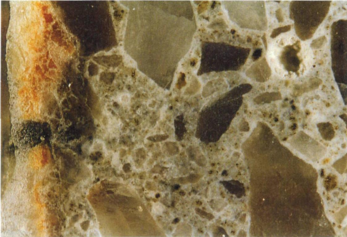
**Image 16:** Corrosion border zone of mortar **K R 1** with limestone and CEM I 42.5 R **MOWILITH-modified**) after 70 days of storage in pH 1 sulphuric acid, ground, under the microscope. The image width is 2.7 mm (55x magnification).
