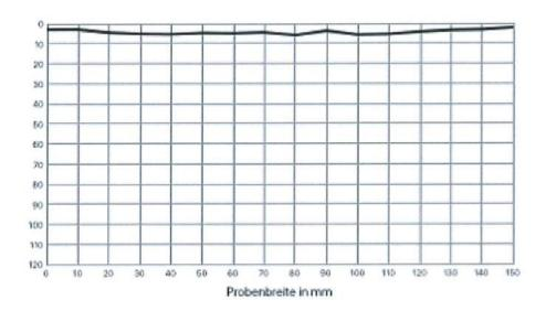
Appendix A1-4: Depth of penetration of water, AD 3000: 2, max. depth of penetration t = 5 mm
