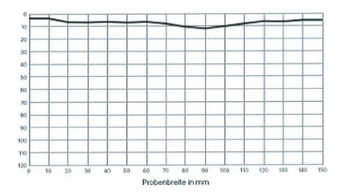
Appendix A1-2: Depth of penetration of water, Reference: 2, max. depth of penetration t = 11 mm
