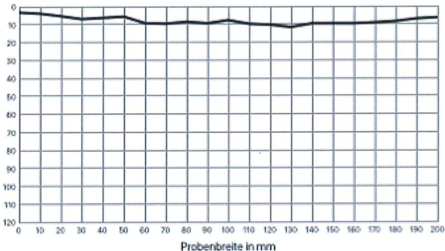
**Appendix A2-3:** Depth of penetration of water, AD 2000: 1, max. depth of penetration  $t = 12 \text{ mm}$
