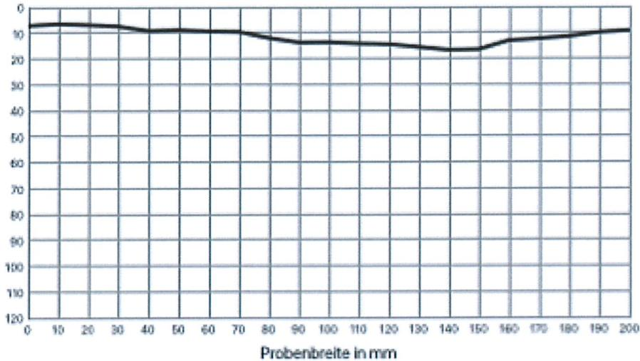
Appendix A2-2: Depth of penetration of water, Reference: 2, max. depth of penetration  $t = 12 \text{ mm}$
